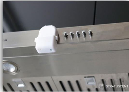
Stratuscent's eNose module installed on the stove hood
